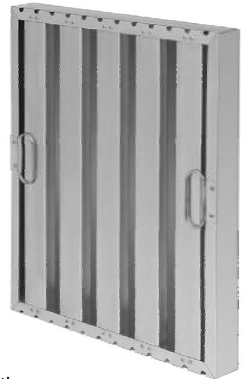
It is universally recognised that there is an increasing need to maintain & improve hygiene standards & reduce fire hazards within kitchens. The Baffle Grease filter accomplishes both needs through it's clever design of interlocking baffles that provide a tortuous route for the passage of air through the filter by creating two rapid 180° air direction changes simultaneously. The grease molecules having a far greater inertial force than air impact themselves on the vanes.
